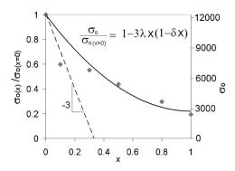
FIG. 6. Pre-exponential factor and normalized pre-exponential factor vs substitution level.
