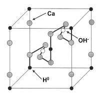
FIG. 7. Hopping path for the conduction mechanism of Ca<sub>12</sub>Al<sub>14</sub>O<sub>33</sub>.
