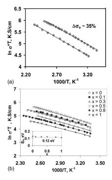
FIG. 5. (a) Arrhenius plot of electrical properties for as-prepared and partially decomposed nonsubstituted mayenite  $(Ca_{12}Al_{14}O_{33})$  from the data in Fig. 2(b). (b) Arrhenius plot of electrical properties for  $Ca_{12-x}Mg_xAl_{14}O_{33}$  (x=0,0.1,0.3,0.5,1).
