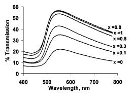
FIG. 8. Optical properties for Ca<sub>12-x</sub>Mg<sub>x</sub>Al<sub>14</sub>O<sub>33</sub>.
