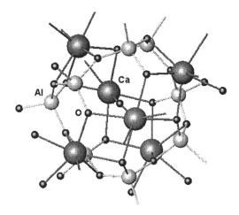
FIG. 1. One of 12 cages constituting the unit cell of  $Ca_{12}Al_{14}O_{33}$ . The charge neutrality is given by the  $O^{2-}$  located inside the cage.
