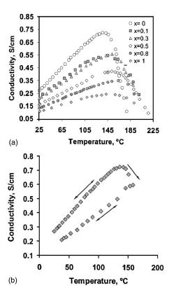
FIG. 2. (a) Conductivity vs temperature of  $Ca_{12-x}Mg_xAl_{14}O_{33}$  (x=0,0.1,0.3,0.5,0.8,1) and (b) conductivity vs temperature of pure mayenite ( $Ca_{12}Al_{14}O_{33}$ ) showing irreversible loss of conductivity above the decomposition temperature (135 °C).
