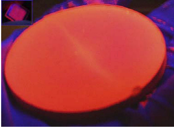
Fig. 2.5. Intrinsic luminescence of wide band gap BaCuSF.
