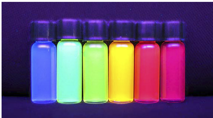
Fig. 1.7. Photoluminescence of colloidal CdSe quantum dots from microwave-assisted reactions at low temperatures.
