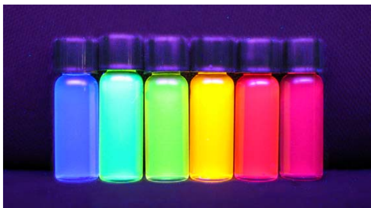
Figure 1.7. Photoluminescence of colloidal CdSe quantum dots from microwave-assisted reactions at low temperatures.
