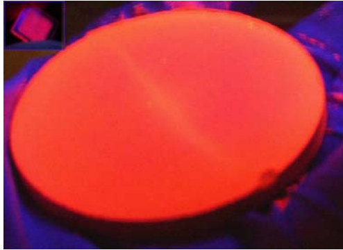
Figure 2.5. Intrinsic luminescence of wide band-gap BaCuSF.
