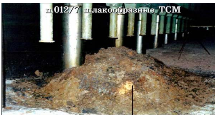
Figure 8.10. “Chemobyl lava,” which primarily consists of the uranyl peroxide Studdite, a naturally occurring mineral that also forms from uranium decomposition in nuclear waste.
